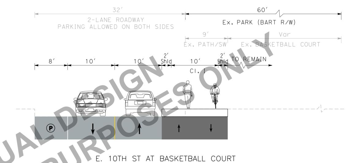
CADD FILENAME **ABBREVIATIONS EAST BAY GREENWAY**  $EBGW\_Railwith Trail\_X-Sections.dgn$ Ex. = EXISTING C&G = CURB AND GUTTER No Scale 02/02/2017 SW = SIDEWALK CONTRACT NO. Rail with Trail LT = LEFT RT = RIGHTTypical Cross Sections DRAWING NO. SHEET NO. R/W = RIGHT-OF-WAYRwT-X12
