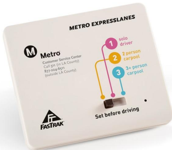
Figure 44: Transponder with Carpool Switch Used in Southern California
